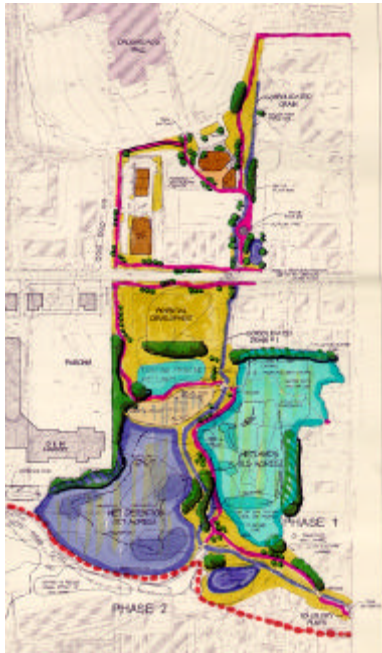
Figure 3. Schematic layout for the new 25-acre innovative stormwater treatment system servicing a 463-acre watershed located in Portage, Michigan.
